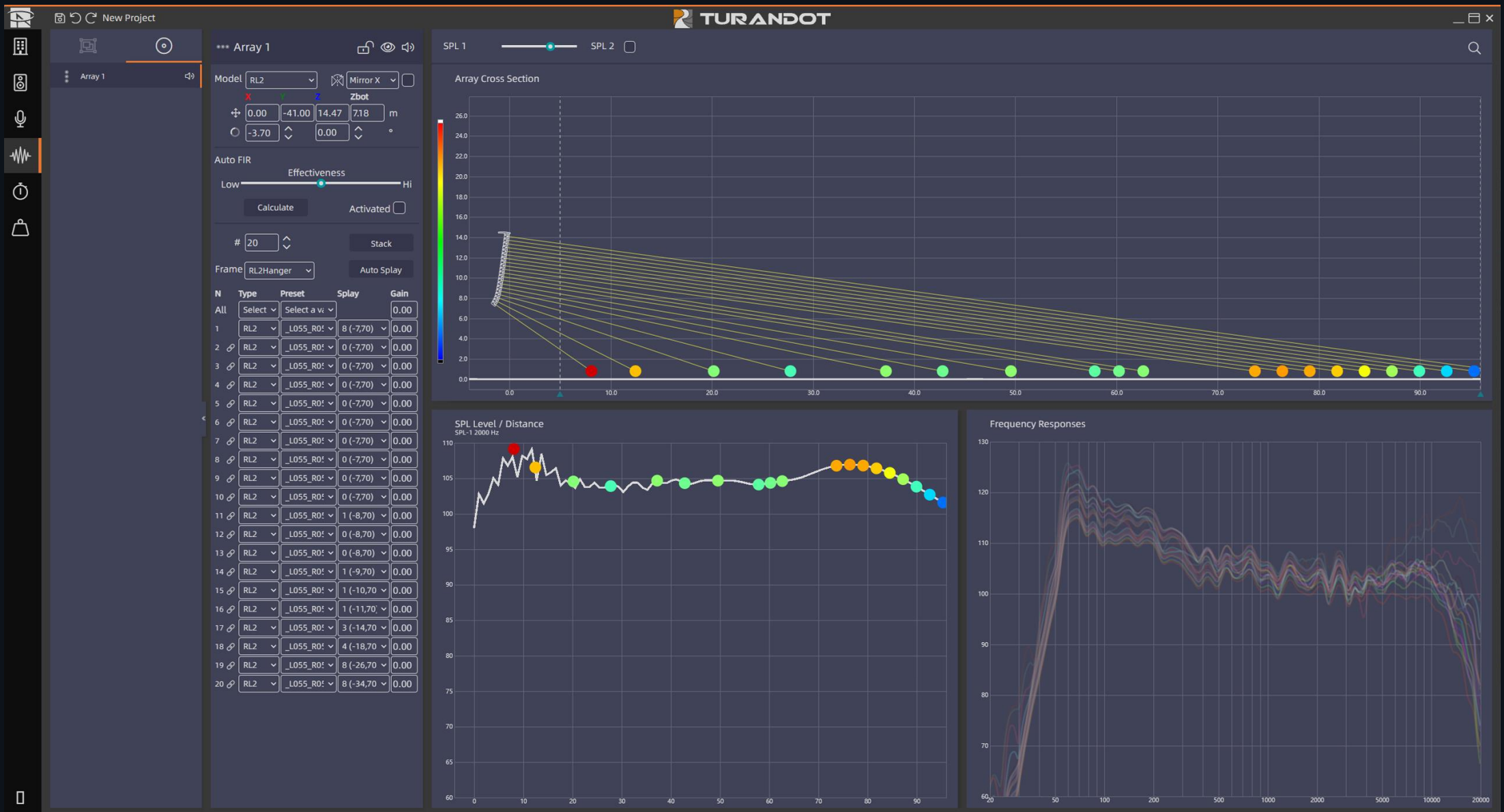
The image shows an example of a created RL2 line array with the speaker cabinet spacing set and the AUTO FIR not calculated or activated.
